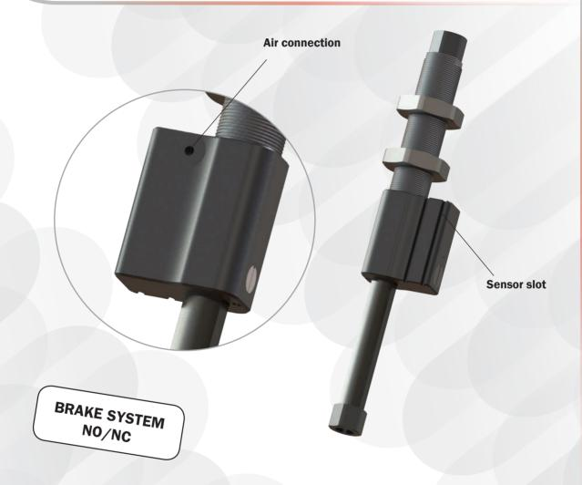
This new smart suspension provides the same features of a standard lever compensator with the additional brake unit that can lock the rod in any stroke position. It can be driven with a single effect pneumatic signal, normally close or normally open depending to the application requirements. The concept, made for high load capability, can be extended to a complete range of suspensions in different sizes and strokes.
